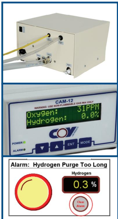
**Track Your Data:** One of the unique aspects of the *Infuser* is the ability to chronicle the oxygen and hydrogen in the chamber through the Data Logging feature. This is ideal for trouble shooting, eliminating errors or to improve chamber efficiency.
